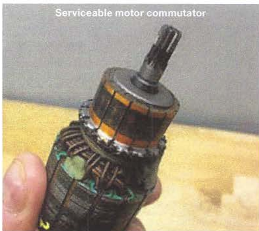
This commutator needs to be turned.
